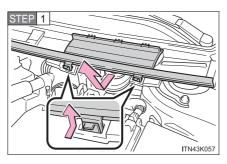
Disconnect the claws to remove the service cover as shown in the illustration.
