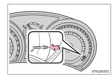
Items displayed can be switched by pressing the odometer/trip meter display change button.
