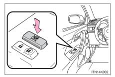
Press the switch down to lock the passenger window switch.
