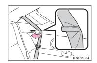
Pass the outboard seat belts through the seat belt hangers.
