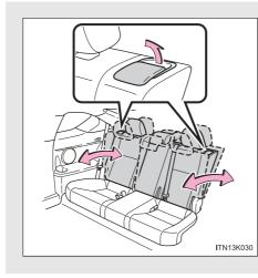
Pull up the seatback angle adjustment lever until the lock is released.
