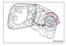
After refueling, turn the fuel tank cap until you hear a click. Once the cap is released, it will turn slightly in the opposite direction.
