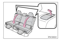
Pull the seatback angle adjustment lever and fold them down.
