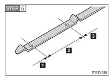
Holding a rag under the end, pull the dipstick out and check the oil level.
