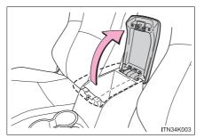
Lift the lid while pulling up the knob to release the lock.
