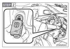
Touch the Scion emblem side of the electronic key to the "ENGINE START STOP" switch.
