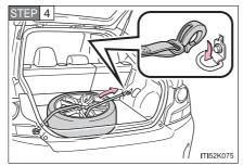
Hook the other end of the belt to the front cargo hook located diagonally to the used rear hook.
