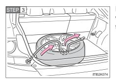
Pass the belts from between the wheel spokes through the center hole of the wheel.
