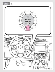
Press the "ENGINE START STOP" switch.
