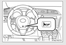
To sound the horn, press on or close to the 🕞 mark.
