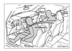
The pretensioners help the seat belts to quickly restrain the occupants by retracting the seat belts when the vehicle is subjected to certain types of severe frontal collision.
