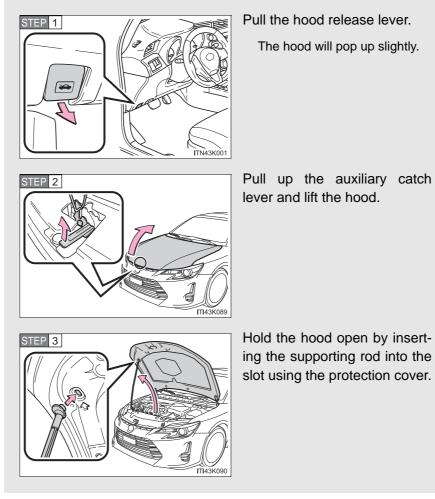
Release the lock from the inside of the vehicle to open the hood.
