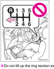
• Do not shift the shift lever to R without depressing the clutch pedal.
