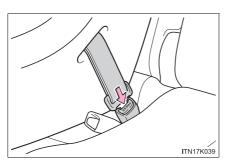
Push the buckle release button and fully retract the seat belt.
