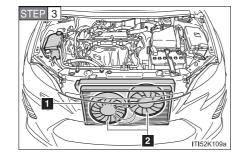
After the engine has cooled down sufficiently, inspect the hoses and radiator core (radiator) for any leaks.
