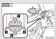
To adjust the mirror, press the switch.
