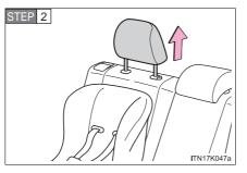
Secure the child restraint system using the seat belt or the LATCH anchors, and adjust the head restraint to the uppermost position.
