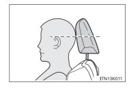
Make sure that the head restraints are adjusted so that the center of the head restraint is closest to the top of your ears.
