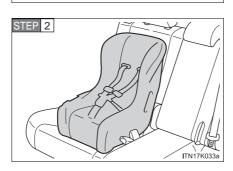
Place the child restraint system on the seat facing the front of the vehicle.
