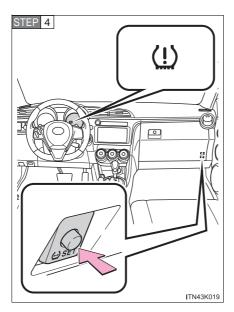
Push and hold the tire pressure warning reset switch until the tire pressure warning light blinks slowly 3 times.
