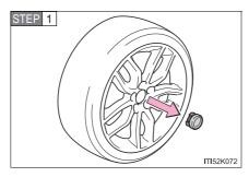
Before stowing the flat tire, remove the center wheel ornament by pushing from the reverse side.
