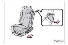
Lift the seatback lock release lever.
