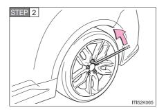
Slightly loosen the wheel nuts (one turn).
