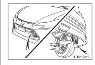
To help enhance safety, install the towing eyelet into the front left hole.
