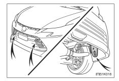
If a tow truck is not available in an emergency, your vehicle may be temporarily towed using a cable or chain secured to the emergency towing eyelet. This should only be attempted on hard surfaced roads for short distances at low speeds.
