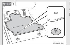
Insert the retaining hooks (clips) into the floor mat eyelets.
