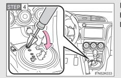
Pry the cover up with a flathead screwdriver or equivalent tool.
