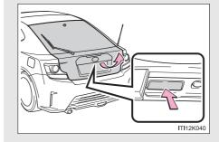
Raise the back door while pushing up the back door opener switch. 1
