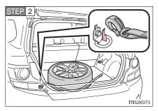
Put the flat tire on the center of the luggage mat with the outer side of the wheel facing up. Hook the end of the belt to either rear cargo hook.
