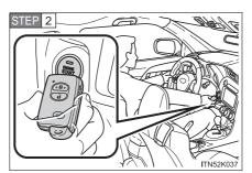
Touch the Scion emblem side of the electronic key to the "ENGINE START STOP" switch.
