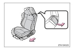
Lift the seatback lock release lever.
