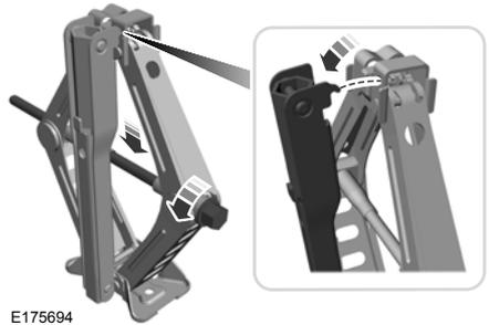
8. To remove the wrench from the jack, turn the hex nut on the jack counterclockwise. This will lower the jack and loosen the mechanical lock.
