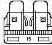
If electrical components in the vehicle are not working, a fuse may have blown. Blown fuses are identified by a broken wire within the fuse. Check the appropriate fuses before replacing any electrical components.
