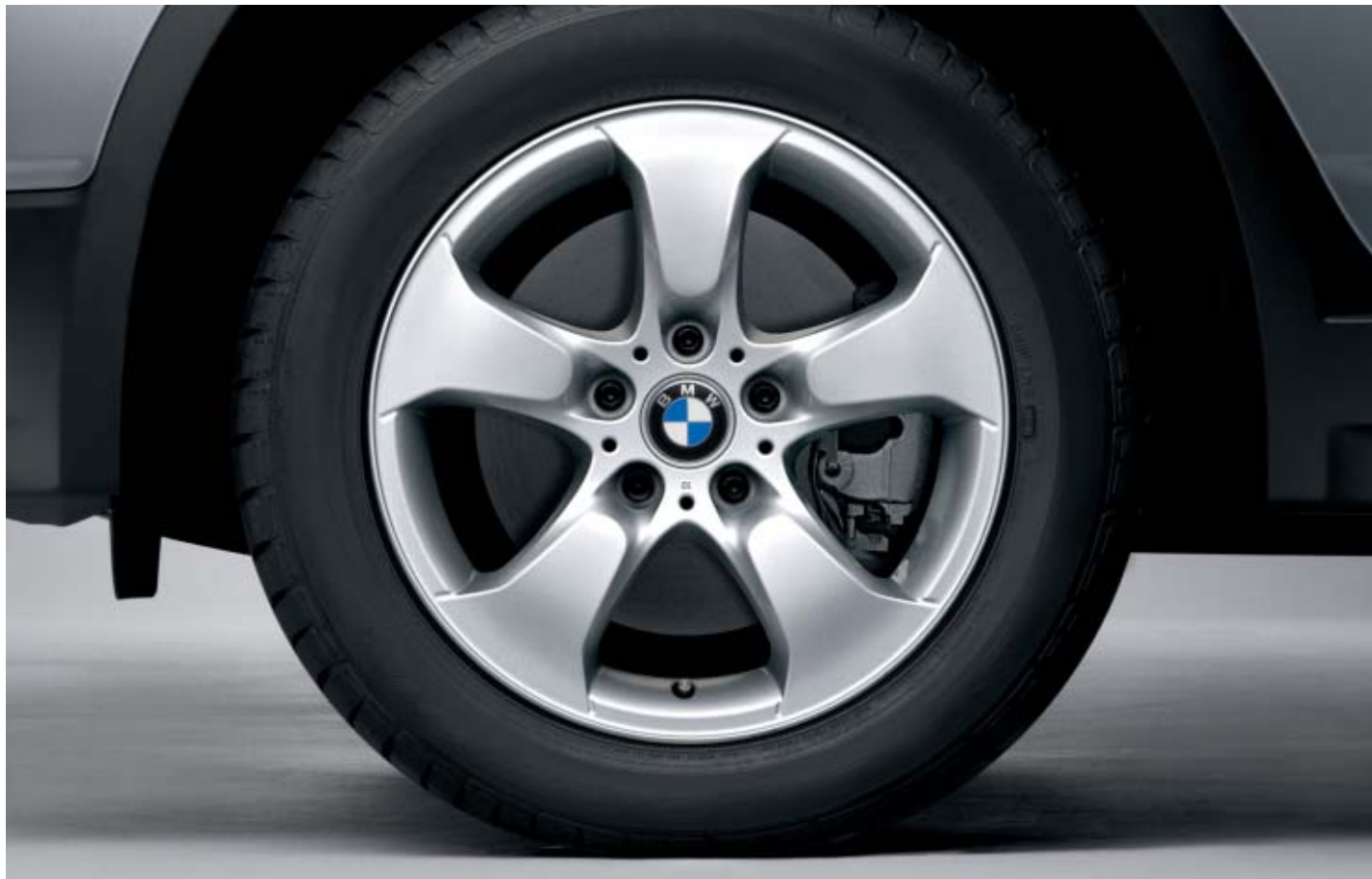
■ 17 x 8.0 Star Spoke (Style 204) alloy wheels and 235/55R-17 all-season tires are standard on the X3 3.0si.
