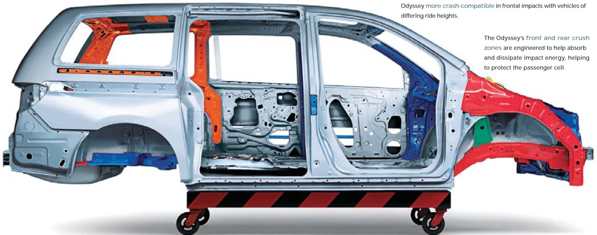
The Odyssey's front and rear crush zones are engineered to help absorb and dissipate impact energy, helping to protect the passenger cell.
